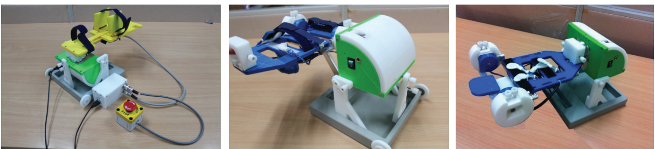
Figure 2. Supporting parts attached to the robot for movements of the elbow flexion-extension (left), for the wrist flexion-extension (middle) and the forearm pronation-supination (right)
