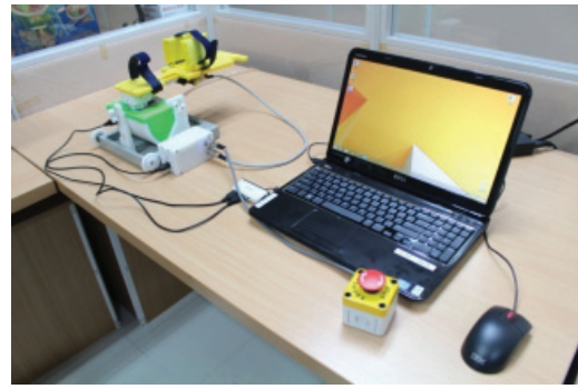
Figure 1. Robot WEFRE rehab system consists of the robot part (on the left), a laptop for setting the programs by therapist and the emergency stop control (red button in front of the laptop)
